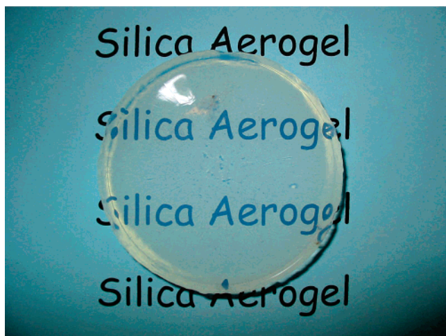
Figure 1. Photo of an aerogel monolite used as a support for Raman experiments lying on a black printed blue paper. The optical transparency allows a perfect reading of the text written on the paper.
